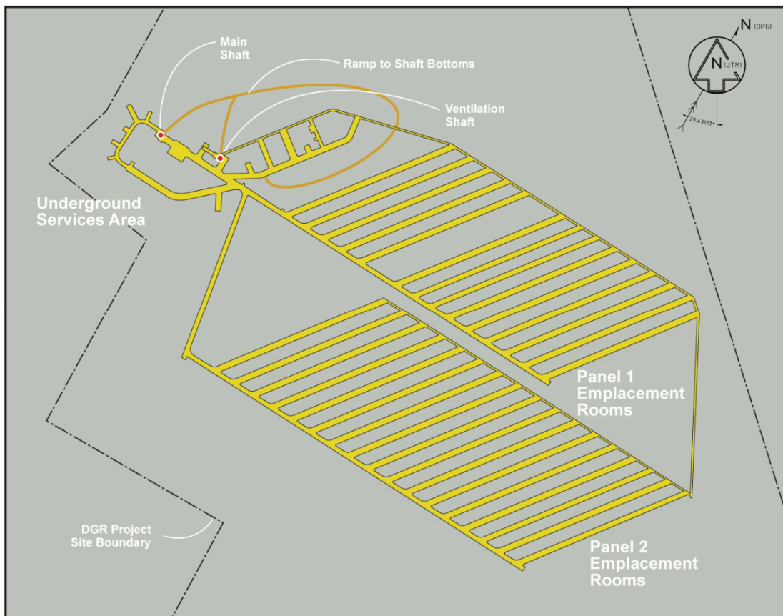
Figure 2.4: Illustration of DGR Underground Facilities
